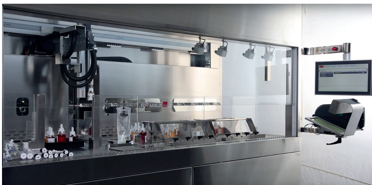
Figure 3: The Equashield PRO fully automated compounding system.
